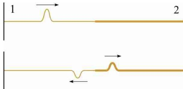
$$v = \frac{d}{\Delta t} \quad \rightarrow \quad \Delta t_{réfl} = \frac{d}{v_1} = \frac{d}{\sqrt{\frac{F}{\mu_2}}} = d \cdot \sqrt{\frac{\mu_2}{F}} = (4 \text{ m} + 4 \text{ m}) \times \sqrt{\frac{0,00275 \frac{\text{kg}}{\text{m}}}{54,5 \text{ N}}} = 0,0568 \text{ s}$$
